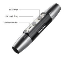
Press the button to turn on the desired function. After switching on, wait about a minute until the UV lamp has reached optimal operating conditions. Pressing the UV button once activates the wavelength of 395nm; a second press activates 365nm. The third press turns off the UV black filter. Pressing the LED button once activates white light, which can be dimmed by pressing it again. Pressing it again turns on warm light, which can also be dimmed. Continuous dimming is possible by long pressing.
